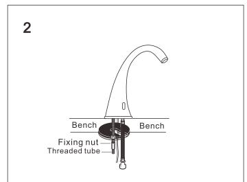
Tighten the fixing nut to secure tap to bench top (do not over tighten as this may damage bench top) Do not tighten the threaded tube.
