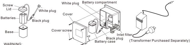
Carefully unplug the black battery plugs, if the battery box cable is pulled the main power white plug can be pulled out from the control box.
