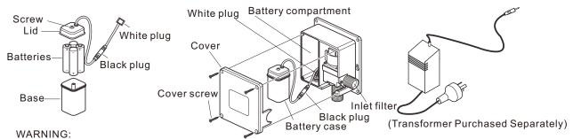
Carefully unplug the black battery plugs, if the battery box cable is pulled the main power white plug can be pulled out from the control box.
