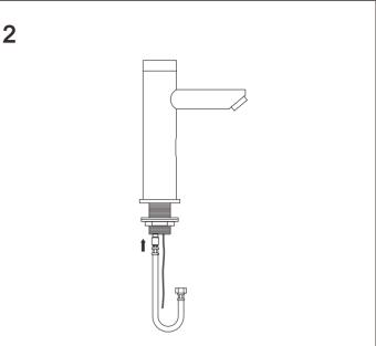
Screw the flexihose on to the bottom of the threaded tube, hand tighten only.
