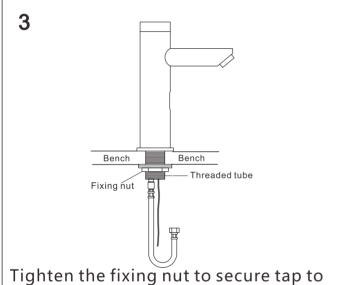
bench top (do not over tighten as this may damage bench top) Do not tighten the threaded tube.
