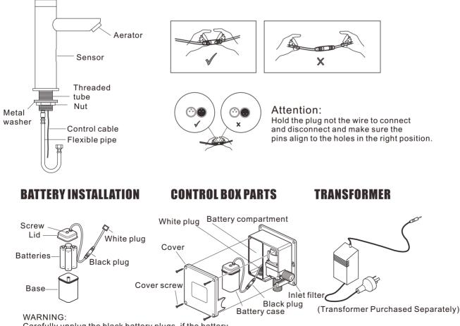
Carefully unplug the black battery plugs, if the battery box cable is pulled the main power white plug can be pulled out from the control box. This will result in the control box not functioning.
