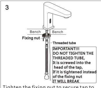
Tighten the fixing nut to secure tap to bench top. (Do not over tighten as this may damage bench top)
