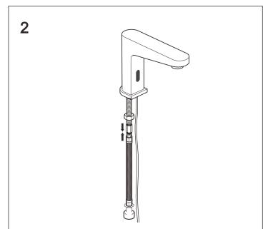
Screw the flexihose on to the bottom of the threaded tube, hand tighten only.
