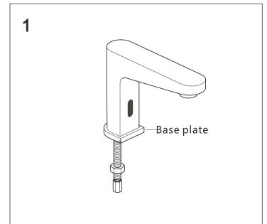
Position the base plate on to the bottom of the tap. (Ensure rubber O-ring is in place)
