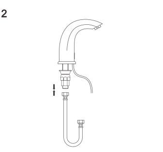
Screw the flexihose on to the bottom of the threaded tube, hand tighten only.
