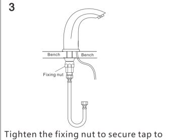
Tighten the fixing nut to secure tap to bench top (do not over tighten as this may damage bench top) Do not tighten the threaded tube.
