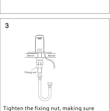
that the baseplate is installed, to
