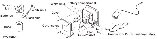
Carefully unplug the black battery plugs, if the battery box cable is pulled the main power white plug can be pulled out from the control box.
