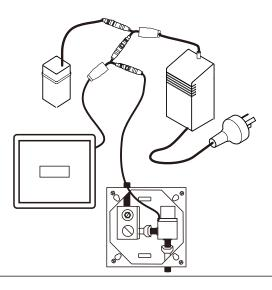
4. Connect transformer to power. Confirm there is power at the socket.
