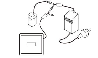
3. Connect solenoid valve to face plate plug.
