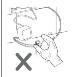
Any operation is disallowed when adapter is connecting to power supply. 100-240V 50-60Hz
