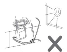
The adapter can't be installed in wet surroundings.
