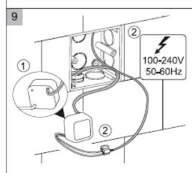
Check if indicator light is bright. If not check if wires are connected to quick connector right. And then check if wires are connecting to power supply normally if all wires are connected right, please contact dealer to repair.
